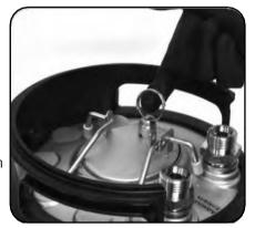
New and regenerated filter media mostly have contaminants. Therefore, the filter should be rinsed twice with the container volume after venting.
