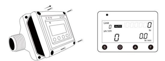
The front case can be rotated from 90, 180 to 270 degree for better reading.
